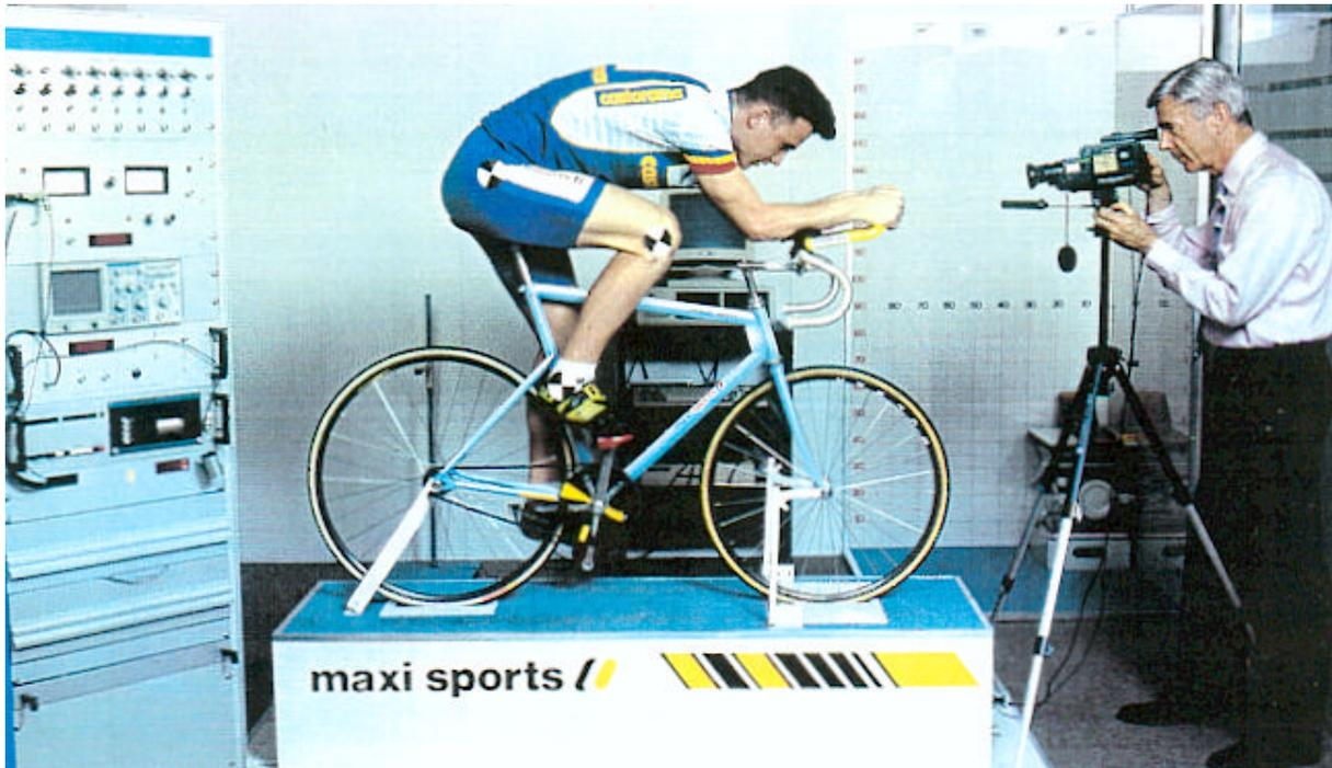
A dynamometric pedal equipped with 8 gauges allowing to measure the torque. The power (torque x angular speed) is non stop put up on a receiver put on the handlebars.
